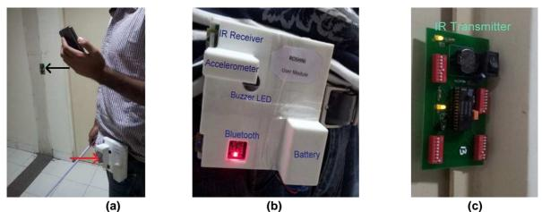
Figure 2: (a) User with the waist worn module (red arrow) and the mobile. Wall-mounted Infrared Unit in background (black arrow) (b) Close-up view of the belt mounted user module (c) a Wall-mounted Infrared Unit
