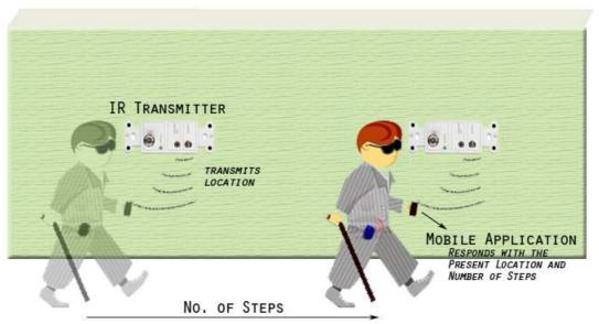
Figure 1: Users get information about the details of their location through mobile application which in turn updates the position of user in the map with the help of IR module (transmits location) and accelerometer (counts the number of steps)
